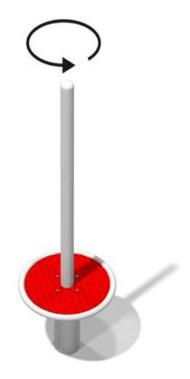
Spinner with diameter 0,3 m. Used components: galvanized steel and PE plate. Thanks to this solution the surface of the device is soft (more safe) and anti-slip. Moreover, it is not heating during sunny days and is not freezing during the winter.
